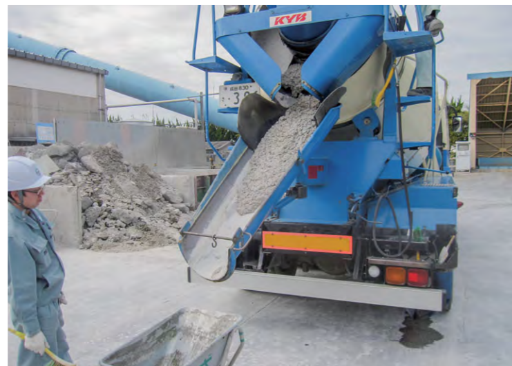
Low-carbon concrete manufactured using by-products from the iron manufacturing process
