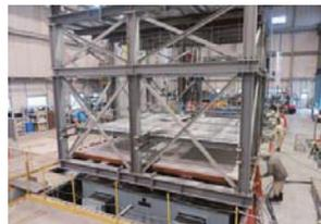
Testing of seismically engineered ceiling clip
