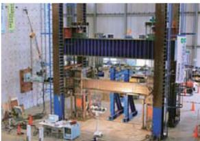
Full-size testing of BiD (built-in damper) construction method
