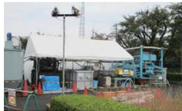
Experimental slurry treatment plant
