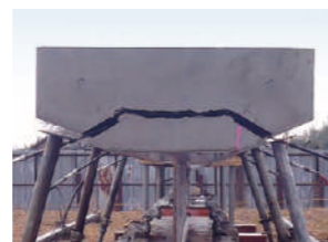
Separation experiment using plate jack
