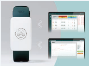
Sigfox Canary and the management screen of its application
