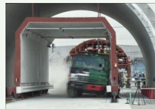
A life-size collision test used to develop the protective work technology
