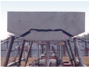
Separation experiment using plate jack
