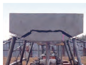
Separation experiment using plate jack
