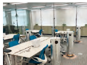
Air-conditioning performance test with simulated load
