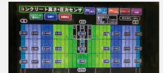
Real-time display of pressure and the height of the concrete pour
