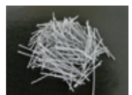
SX20 Fiber diameter 0.37mm× fiber length 20mm
