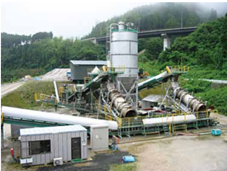
Full view of a CRT mixer system
