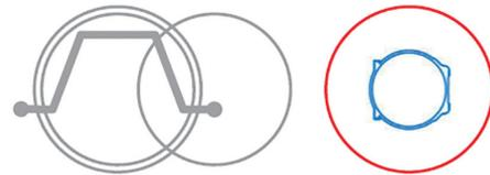
2. Pre-auger (先行削孔) φ685mm
